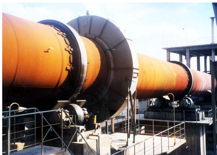
Open gearing, such as this huge ring gear that drives this rotary cement kiln, pose special lubrication challenges ... SWEPCO 164 Open Gear EP Grease solves them.
